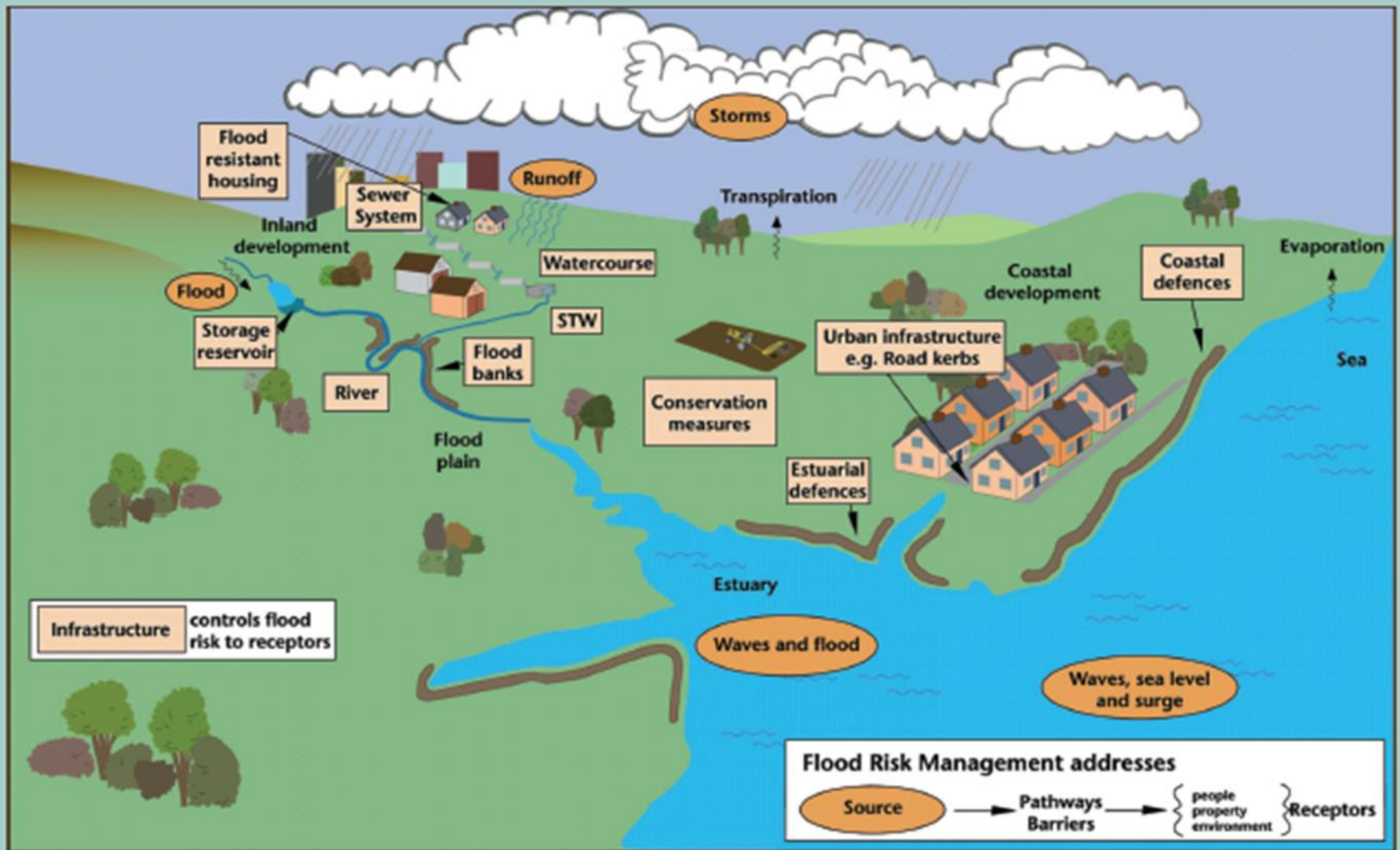
Sources and pathways of flooding, and the receptors at risk
